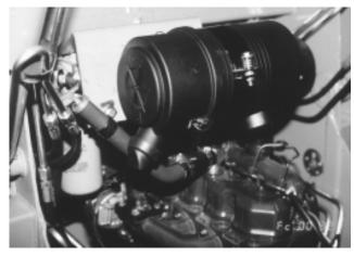
Despite its compact size, the FPG Air Cleaner offers complete engine air protection – removing 99.99+% of the dust and dirt particulate that enters the engine airstream.
