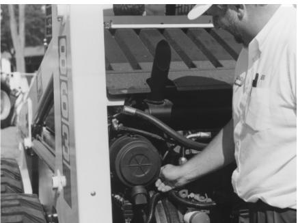
FPG Air Cleaners, with RadialSeal™ Sealing Technology, provide thorough two-stage cleaning of incoming engine air on industrial and construction vehicles operating in medium to heavy dust environments.
